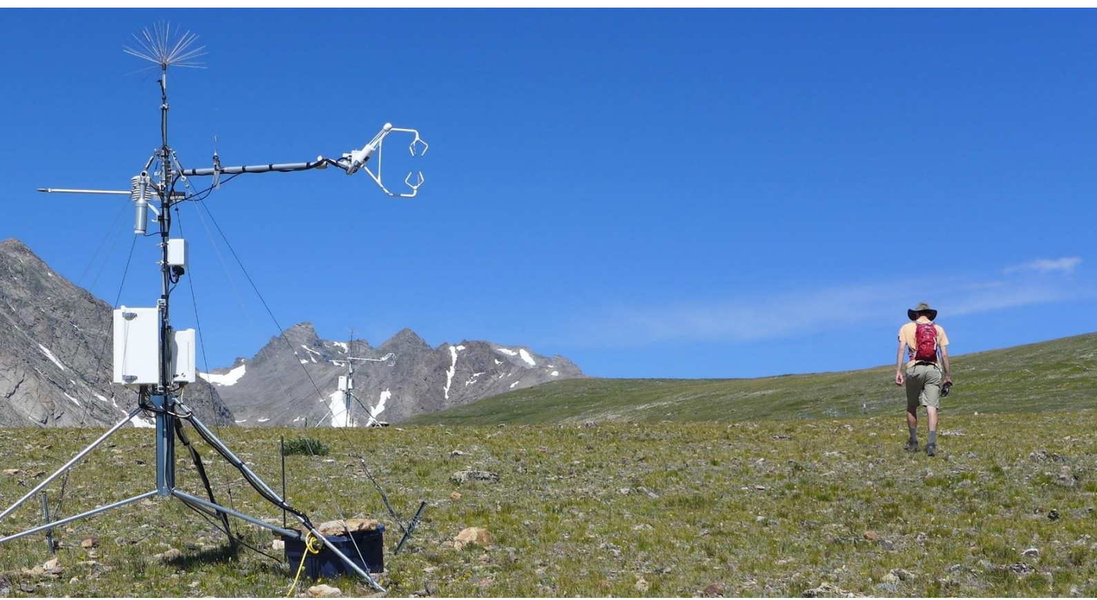
Figure 3: Each study site (right) is equipped with a micrometeorological flux tower (above). Each tower takes near continuous measurements of CO 2 flux and various meteorological variables. Only data from the summer months were analyzed in this study.
